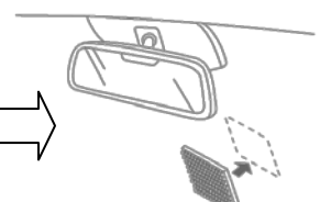
Fix the adhesive side of the 3M velcro on the selected location. Apply pressure on tape for > 30 seconds. Wait for at least 1 hour before using it.
