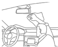
Select & clean the windscreen area before mounting the Recorder
